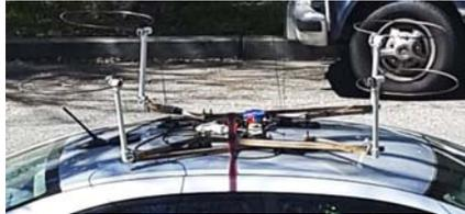
**Fig. 4 HF Doppler DF array using four small horizontal loops and 2m DF vertical sticks**
