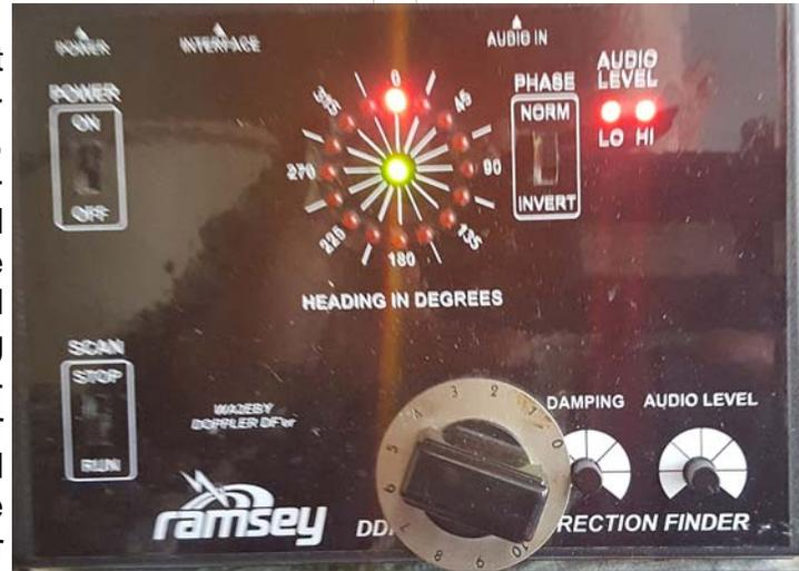
Fig. 1 Ramsey Electronics Doppler Direction Finder, DDF-1
