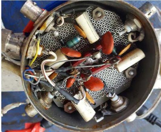
**Fig. 8 Antenna switching circuit in tuna can (antennas disconnected, turned upside down)**
