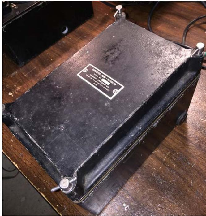
**Fig 1 T-894 with the top cover which closes the transmitter tightly sealed with a gasket.**
