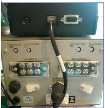
The rear apron has a DB-9 serial to connect controller to computer and RJ-45 connector for the rotator. Obviously, rotators for a satellite ground station have to rotate in elevation and Azimuth. XOX-TRAK used the RJ-45 which you can find anywhere from the LAN cable and on the other end will have 8 pin Din type connector already made up compatible with Yaesu Model G5400,G5500 and G5600.
