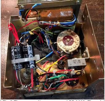
Fig 5 The restored/reconstructed PP-2685. There is a silicon bridge rectifier on the right bottom.
