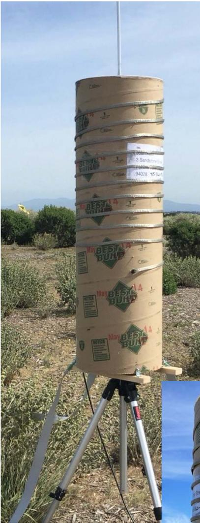
This odd looking thing is actually a pretty efficient 40-10 meter center-loaded high-Q vertical antenna made of a contractor's cardboard tube that was left over from my house remodeling project. I had a SSB QRP QSO with a W9 station on 40m from Palo Alto's Baylands Open Preserve.
