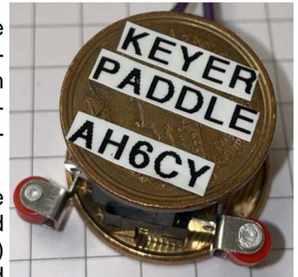
You may have noticed the lead wires (and plugs) are repurposed free earbuds that airlines give out on long distance flights. The round bases are repurposed metal pieces I picked up at flea market for pennies. I have no idea what they were originally for.
