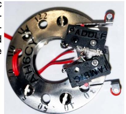
This one is made with two repurposed foreign coins sandwiching two micro-switches.
