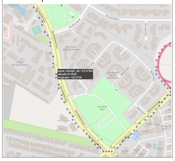
Users can mouse-over the samples and the signal strength and lat/lng location show up in a tooltip. These interactive maps work just like google maps, and can pan/zoom easily. The error and timestamp are recorded in the map as well but don't show up in the tooltip by default.
