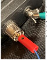
I brought out my portable rig, shoved one end of a short wire into the center of the tuner antenna connector, clipped the other end to my downspout, and made sure I had metal-to-metal contact. Then I threw a
