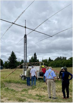
The antenna party crew is checking the SWR of the 40M mono band antenna in preparation for Field Day.
